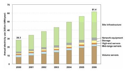
**Figure 1:** Data Center and Server Efficiency (Source EPA)
