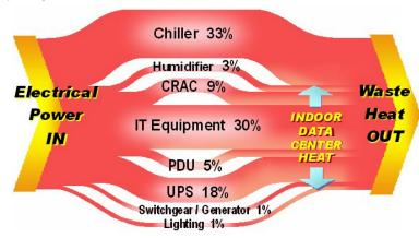
**Figure 2:** Electrical Efficiency in a Data Center (Source: APC)
