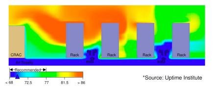
**Figure 3:** Air Flow in a Traditional Data Center
