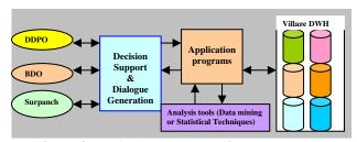
Figure 3: Typical components of VEDP-DSS
