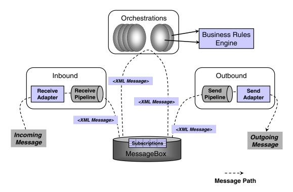
Figure 4: Main Components of the Engine
