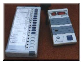
Figure 1: Electronic voting machine & control unit
